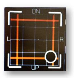
position indicator shows that, in fact, the pilot did the opposite; pulled the stick all the way aft and all the way over to the right. This is archetypal unhelpful behaviour: not simply a failure to do the right thing, but *actively* doing the wrong thing.
